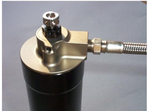
When installing the shock or strut on the car for the first time, the LSC adjuster (the small knurled knob) should be set at minus 15 clicks from "Full Stiff" and the HSC adjuster (the ½" hex knob) should be set at 6 clicks from "Full Soft". This is a good place to start, "mid range".
