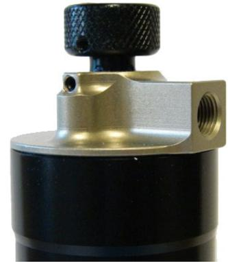
When installing the shock or strut on the car for the first time, the Compression adjuster (the knurled knob) should be set at minus 12 clicks from "Full Stiff". This is a good place to start, "mid range".
