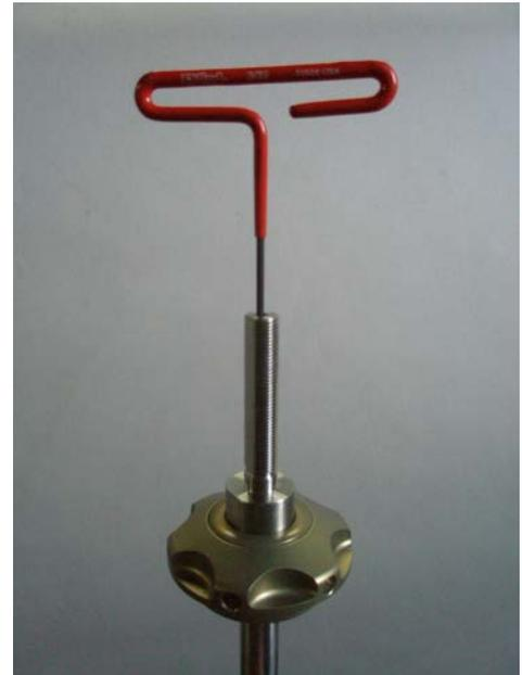
When installing the shock or strut on the car for the first time, the REB adjuster should be set at minus 2 full turns or minus 8 quarter turns, from “Full Stiff”. This is a good place to start, “mid range”.
