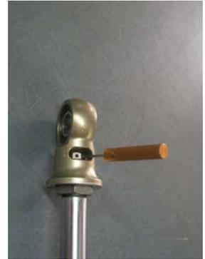
When installing the shock or strut on the car for the first time, the REB adjuster should be set at minus 12 sweeps from “Full Stiff”. This is a good place to start, “mid range”.
